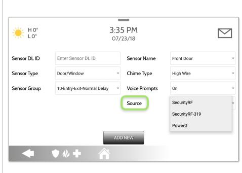
Source indicates the sensor's incoming frequency when pairing to the IQ Panel 2 and IQ Panel 2+.
