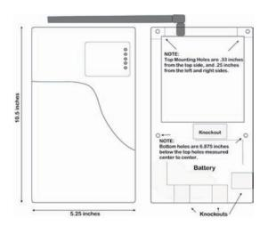
FIGURE 2: Inside & Outside Mounting Dimensions for the 4530
