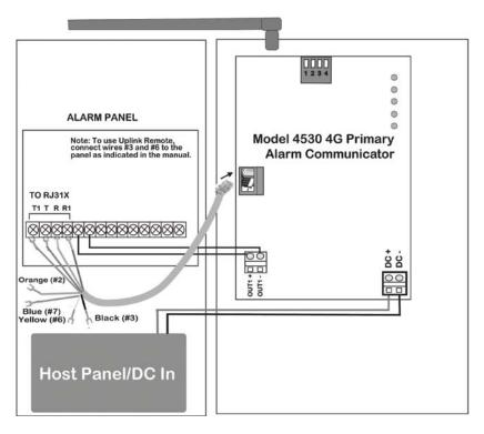
FIGURE 3: Connections between the 4530 and the Alarm Panel
