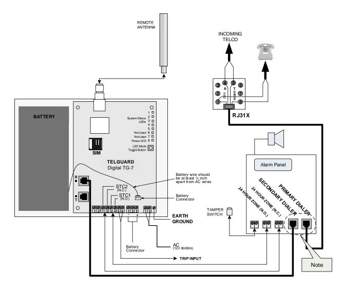
Note: When using this scheme, the use of the primary or secondary dialer to connect to Telco is what determines whether the TG-7 is meant to work as a back-up or primary communicator.
