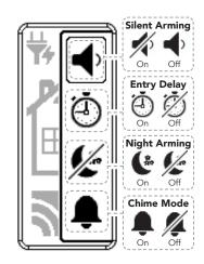
**Change HeliPad settings** using the extended menu. Hold **MENU until** the HeliPad chirps three times (roughly 3 seconds) to open the extended menu.
