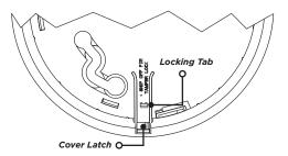
Figure 4: Mounting Base and Tamper Switch
