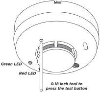
Figure 6: Test Button Location
