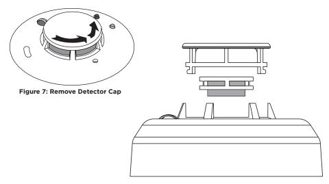
Figure 8: Detector Cover and Sensing Chamber
