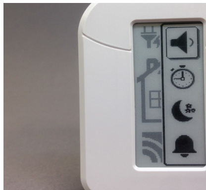
Features can be modified for each arming session. The settings remain static between arming, and can vary between HeliPADs on the system.
