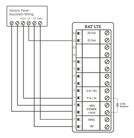
For basic keyswitch interactive services with the BAT LTE, the following alarm panel wiring is needed.
