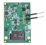
The 2GIG-LTEV-A-GC3 is a 4G LTE radio for the Verizon network to work with Alarm.com. This new radio transfers both data and two-way voice over Verizon's 100% LTE network and VoLTE (Voice over LTE) technology.
