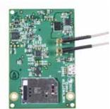
The 2GIG-LTEV-A-GC2 is a 4G LTE radio for the Verizon network to work with Alarm.com. This new radio transfers both data and two-way voice over Verizon's 100% LTE network and VoLTE (Voice over LTE) technology.
