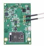
The 2GIG-LTEV1-NET-GC2 is a 4G LTE radio for the Verizon network to work with SecureNet. This new radio transfers both data and two-way voice over Verizon's 100% LTE network and VoLTE (Voice over LTE) technology.
