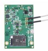
The 2GIG-LTEV1-A-GC2 is a 4G LTE radio for the Verizon network to work with Alarm.com. This new radio transfers both data and two-way voice over Verizon's 100% LTE network and VoLTE (Voice over LTE) technology.
