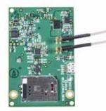
The 2GIG-LTEV1-A-GC3 is a 4G LTE radio for the Verizon network to work with Alarm.com. This new radio transfers both data and two-way voice over Verizon's 100% LTE network and VoLTE (Voice over LTE) technology.
