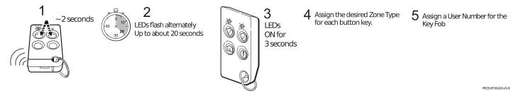
**NOTE**: Once enrolled in a system, the PROSiXFOB cannot be used with another controller until it is removed from the current controller. When removed from a system, the key fob will revert to factory default settings.
