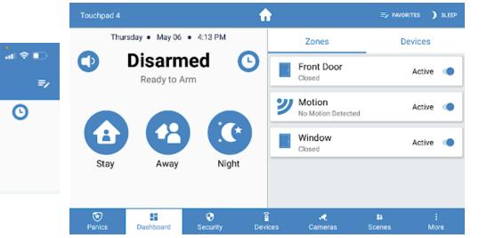
The **Clock Icon** performs an instant arm function. When using this function, any zone opened when the system is armed will trigger an alarm instantly, without an entry delay.
