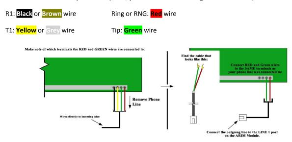
IF your existing phone line is still connected to the panel, make note of which terminal connectors the RED and GREEN wires are connected to. Then disconnect **ALL FOUR** Wires of the phone line from the panel. Then connect the RED and GREEN wires from the cable we sent with the ARIM to the same connectors for RED and GREEN that your phone line used.
