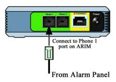
If you need a longer cable for this connection, you may lengthen the cable provided by using an in-line adapter, which can be found at most electronics stores, and a second, regular phone line (like the ones used from your phone jack to your phone). The total length of cable, from the panel to the ARIM module, CANNOT EXCEED 25 FEET. Cables longer than 25 feet reduce the strength of the alarm signal, and prevent AlarmRelay from getting clear signals from your alarm panel.
