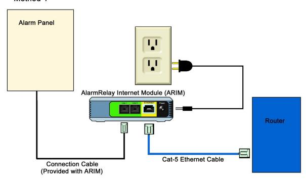
If distance or structure prevent you from running a straight Cat-5 Ethernet cable connection from the ARIM to your Router, there are other methods of connecting. Please refer to the document "ARIM Module: Other Connection Methods.pdf", which you can download from:
