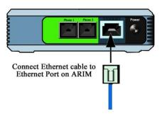
If the provided cable is not long enough for you, you will have to provide your own cable that is long enough. Total Ethernet cable length CANNOT EXCEED 300 FEET.
