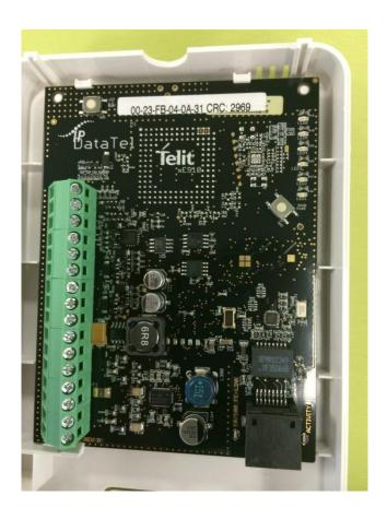
**NOTE:** As you can see there are 16 screw terminals adjacent to the left side of the board. We will be wiring from this board to the alarm panel circuit board later on in this guide.
