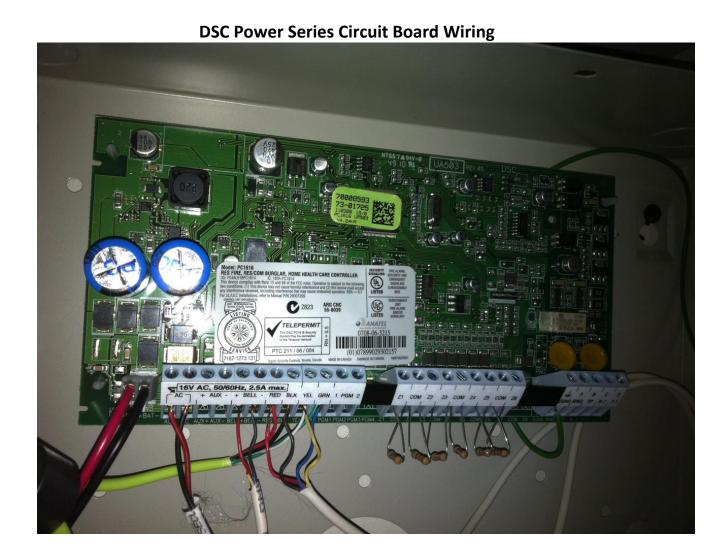
As you can see, this panel has about 25 screw terminals on the bottom of the board. Using the cable with the 4 different color wires on each end you will wire up to the panel as follows (refer to pg. 15 for diagram):
