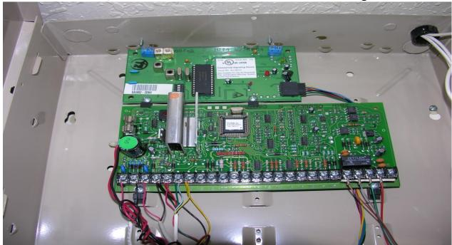
As you can see on the Vista panel there are about 25 screw terminals along the bottom. You will take the cable that has 4 different colored wires (red, black, green, and yellow) exposed on each end and screw them in to the terminals in the following order (**Refer to pg. 14 for diagram**):
