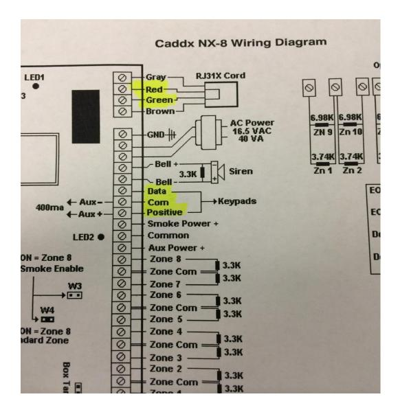
As you can see, the terminals we need to connect to on this system circuit board are Data, Com, Positive, Red, and Green. Sometimes, they are labeled KP Data, KP Com, and KP Positive as well. You will wire the cable with the 4 wires on each end (red, green, black, and yellow) to this panel (refer to pg. 16 for diagram).
