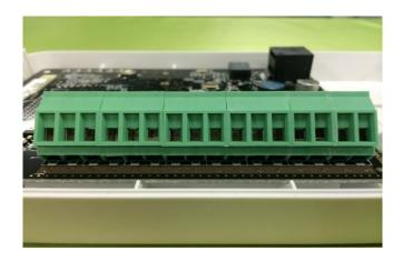
NOTE: The wires need to be inserted through the square shaped holes (terminals) that are part of the green terminal strip. The screws should already be loosened so you will just need to tighten them.
