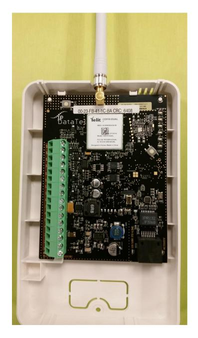
**NOTE:** As you can see there are 16 screw terminals adjacent to the left side of the board. We will be wiring from this board to the alarm panel circuit board later on in this guide.
