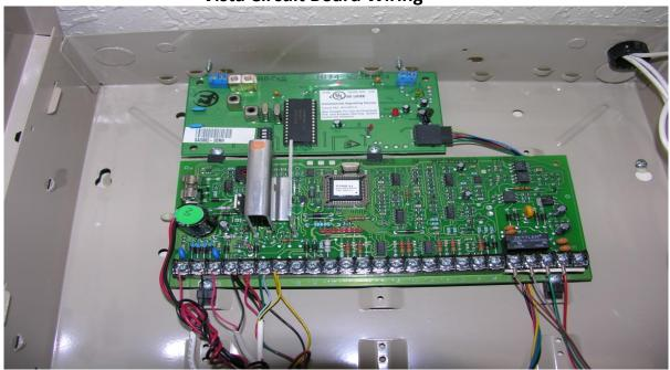
As you can see on the Vista panel there are about 25 screw terminals down the bottom. You will take the cable that has 4 different colored wires (red, black, green, and yellow) exposed on each end and screw them in to the terminals in the following order (refer to pg. 13 for diagram):
