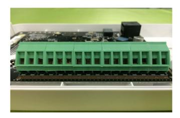
NOTE: The wires need to be inserted through the square shaped holes (terminals) that are part of the green terminal strip. The screws should already be loosened so you will just need to tighten them.
