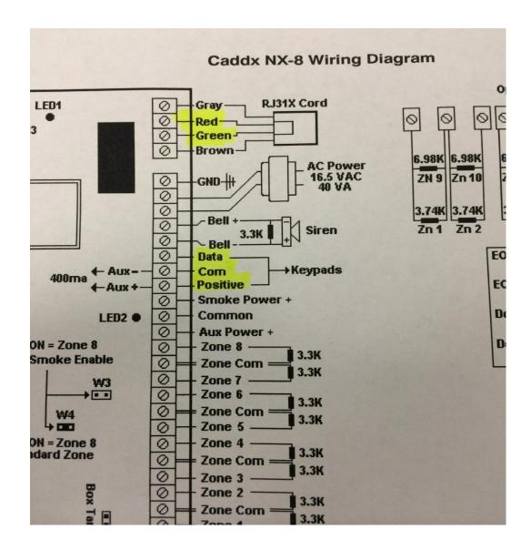
As you can see, the terminals we need to connect to on this system circuit board are Data, Com, Positive, Red, and Green. Sometimes, they are labeled KP Data, KP Com, and KP Positive as well. You will wire the cable with the 4 wires on each end (red, green, black, and yellow) to this panel (refer to pg. 15 for diagram).
